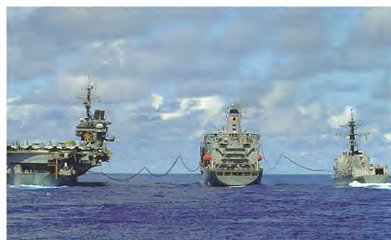
The USS Kitty Hawk being refueled by the USS Platte. On the right is the destroyer USS Elmer Montgomery.
